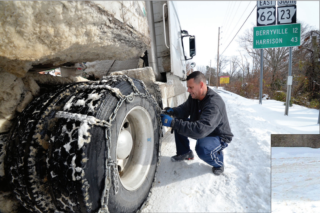
Chains, chains, chains – These chains fooled Jason Simmons of Reliable Trucking by spinning loose while ascending Planer Hill on Saturday. Eighteen-wheelers cannot pull over onto the shoulder safely in this area so Simmons, like many other truckers this past weekend, was forced to stop on US 62 to make adjustments and tighten the chains on his rig.
